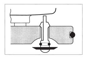
The plastic seals tightly against the cylinder by means of a rubber gasket. The plastic air valve itself can be easily removed for cleaning by light pressure from above. The polished inside of the cylinder ensures smooth turning of the cranks and easy cleaning.
