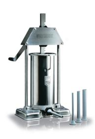
These sausage fillers are available in three sizes (9, 12 and 15 litres), of sturdy construction, easy handling and especially hygienic. Gear box, toothed and lateral rack, cylinder, base plate with cylinder holder as well as the crank are made of stainless steel and meet the highest quality demands. Second gear for fast return speed of piston.
